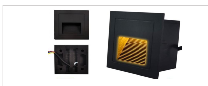
IP65 Square recessed wall light GR-BD-L-03 / 3W 100-240VAC 50/60Hz L86*W86mm, Cutout: 80*80mm
